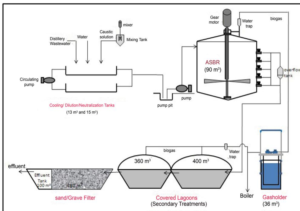
Figure 5. Design of full-scale distillery wastewater treatment plant.
