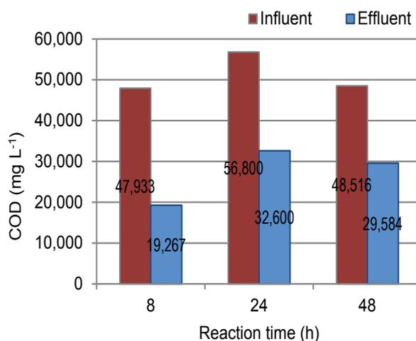
**Figure 3.** COD values in influent and effluent after ASBR operation with different reaction time. Data in ASBR with 8 h reaction time was based on 7<sup>th</sup> day operation. Data are means from two trials.
