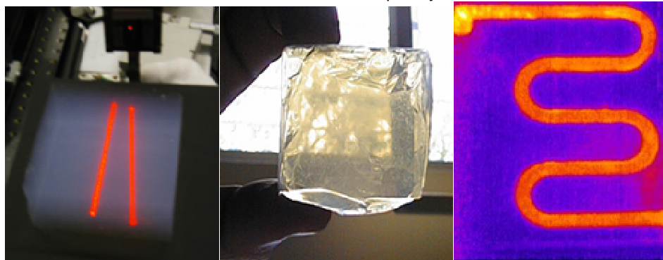
Figure 1. The laser beam crosses twice the aerogel [1]. A piece of silica-aerogel which was used to perform self-measurements [5]. IR-snapshot of an \text{AlSi}_7\text{Mg}_{0.5} meander casted in pure silica-aerogel molds 6 sec after completely filling the mold. The meander is 5 mm thick [3].
