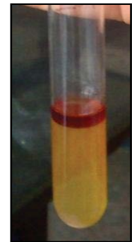
Figure 2A. Indole test: When kovac’s reagent (p-dimethylaminobenzaldehyde) was added to the broth with indole in it, a dark pink colour developed.
