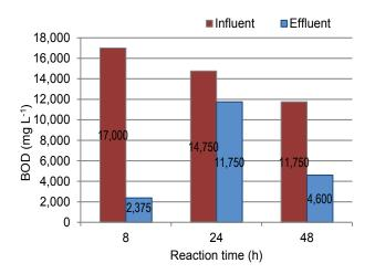
**Figure 4.** BOD values in influent and effluent after ASBR operation with 8 h, 24 h, and 48 h reaction time. Data in ASBR with 8 h reaction time was based on 7<sup>th</sup> day operation. Data are means from two trials.
