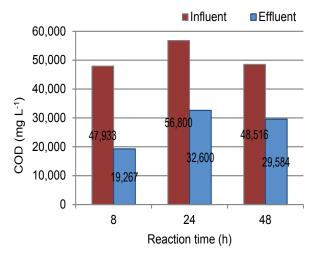
**Figure 3.** COD values in influent and effluent after ASBR operation with different reaction time. Data in ASBR with 8 h reaction time was based on  $7^{th}$  day operation. Data are means from two trials.
