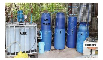
**Figure 2.** Fabricated ASBR and biogas holders. Capacity: ASBR, 1,000 L; gas holders, 245 L.
