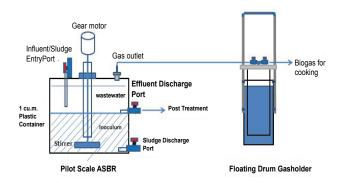
**Figure 1.** Schematic diagram of the pilot-scale anaerobic sequencing batch reactor (ASBR) system.
