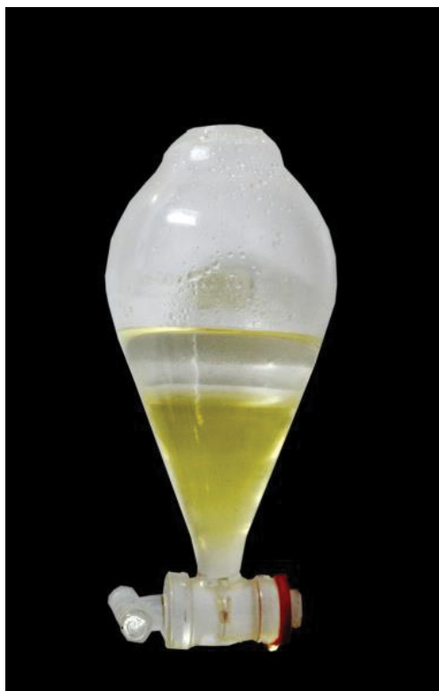
Figure 2. Separation of metabolites using separating funnel: upper layer contains metabolites in ethyl acetate.
