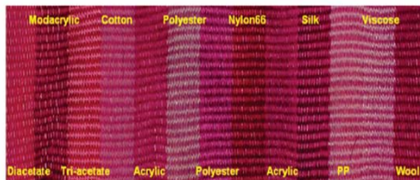
Figure 4. Colored multifibers fabric with the red pigments from Vibrio spp. Strain KSJ45, [112].
