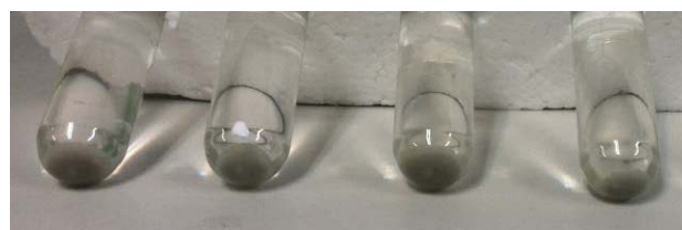
Figure 1. Formation of black precipitate during bioreduction experiments using isolated bacteria.
